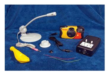
Shown above is a kit from Quaketronics.com. Included is a microphone which is plugged into the black trigger control box on the right. Other miscellaneous parts are used to convert that Kodak camera into an inexpensive remotely triggerable high-speed flash, which is also plugged into the trigger control box.
